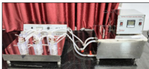
6 Stage Franz Diffusion Cell Apparatus, Orchid Scientific
